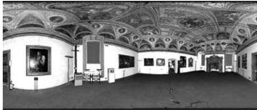
Figure 6.1. "Sala del Camin Nero"- Castello Buonconsiglio, Trento: reflectance image of a single scan acquisition acquired in 3 min and 22 sec.
